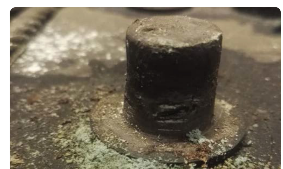
Damaged, scratched & indented terminal post. Excessive dirt build up from lack of battery care & maintenance
