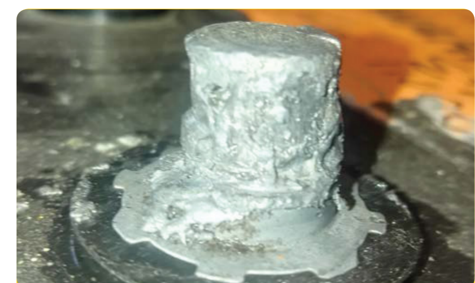
Melted terminal post caused from extreme heat.
