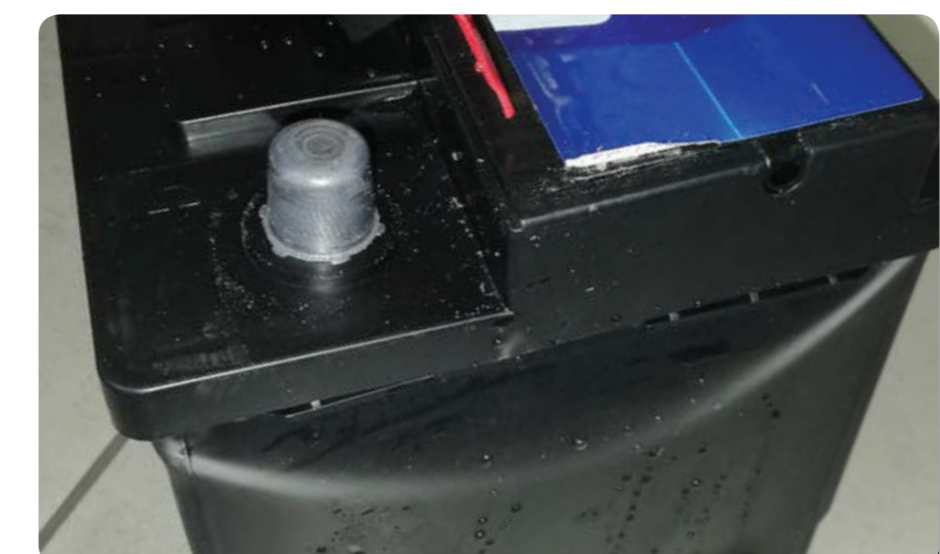
Damaged Battery casing indented.
