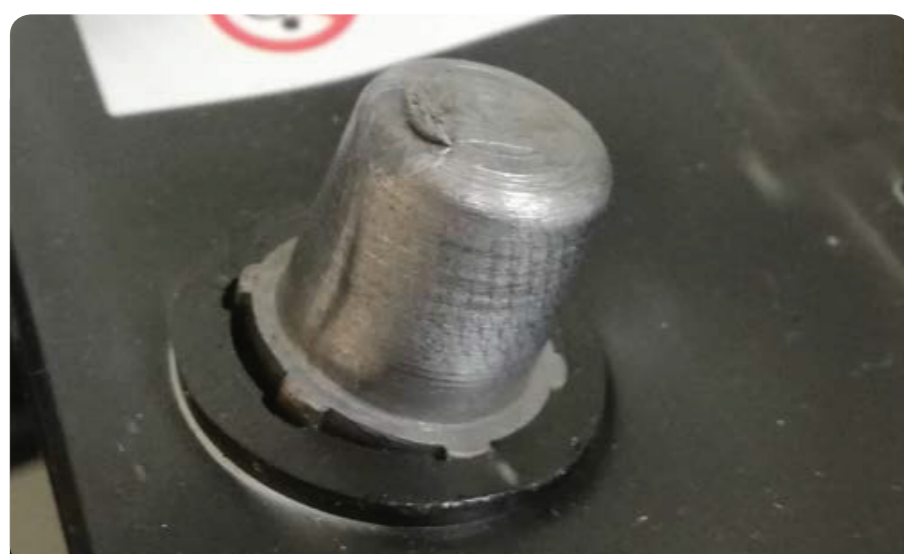
Bent terminal post caused from the use of excessive force.
