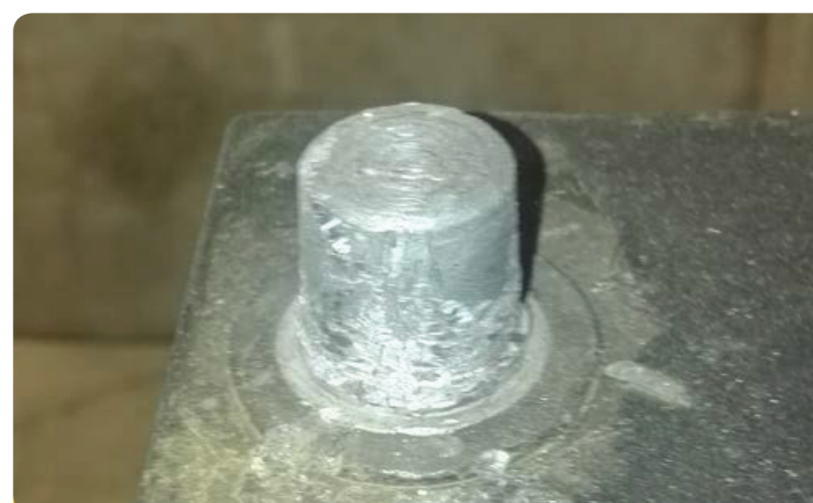
Indent on terminal post damage caused from over tightening post clamp resulting in poor connection.
