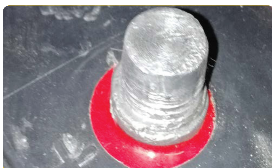
Damaged terminal post.
